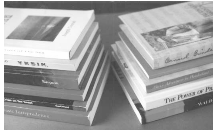
Book Stacks. Books from large and small book-on-demand systems. Can any of these practitioners get the total cost for a 300-page book down to about $5? Books in the left-hand stack are not laminated and exhibit some wear at the corners; at the right are laminated books, with minimal wear.
